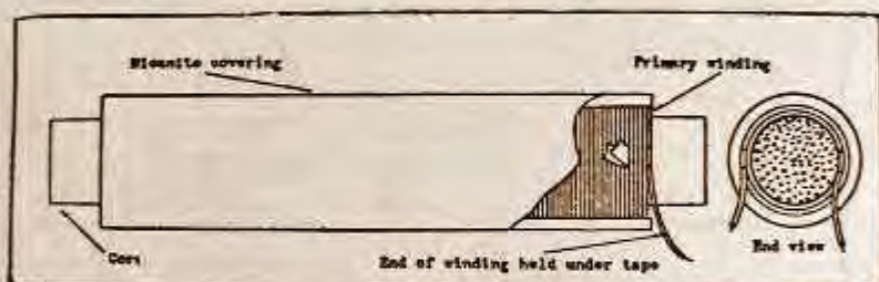
Fig. 29.—Core and primary, showing how finishing end of primary winding is held under a loop of tape.
