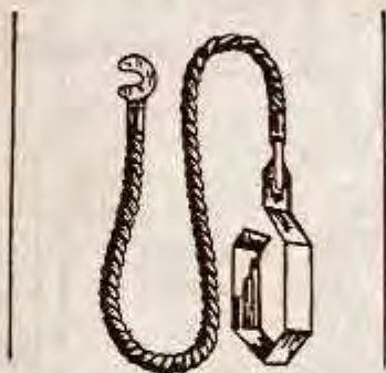
Fig. 105.—Spring connector and cord for condenser
