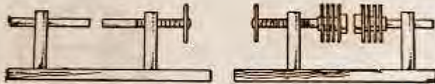
Fig. 14.—Designs of stationary spark gaps. The type at the right is fitted with rotating discs to dissipate the heat generated by the spark
