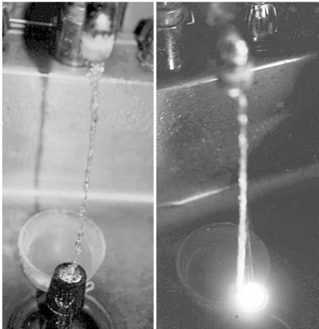
Flashlight experiment illustrating photonic waveguide effect.
